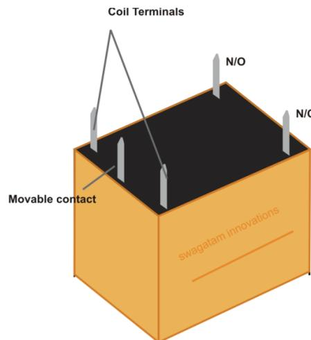
Relays are switches that open and close circuits electromechanically or electronically. They control one electrical circuit by opening and closing contacts in another circuit. When a relay contact is normally open (NO), there is an open contact when the relay is not energized.
